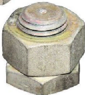
Figure 2 - Thin nut placed next to the joint.
